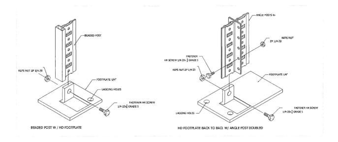
Here is when the installer needs to make sure that all the datum lines match the footplates/posts locations, and check for uneven surfaces to compensate using shims under the footplates.
