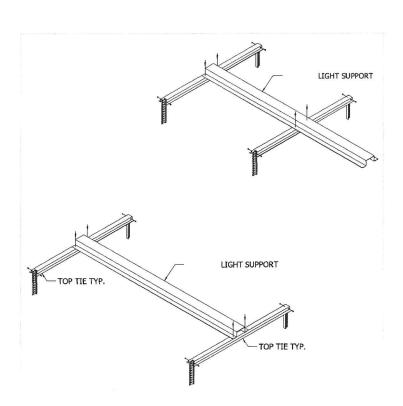
The light support overhang, over the tie support, is used to hang lights at the end of the sections, where no more shelving units are present.
