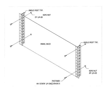
Back Panels must be installed in a "tucked fashion", meaning that the lower back panel should always overlap the upper back panel. See the details below.
