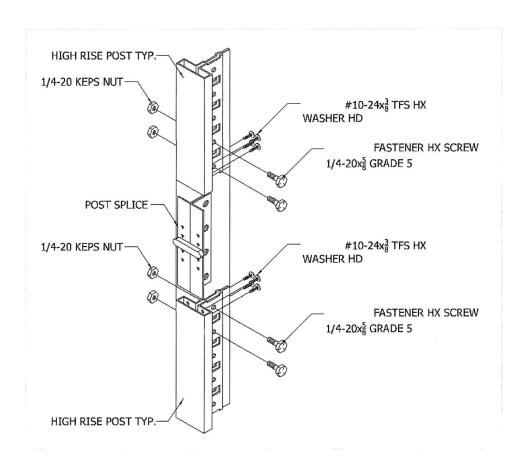
The beaded post splicer consists of steel plate welded at right angles to a front plate, which is attached with self-threading screws. It also includes a splicer bar.
