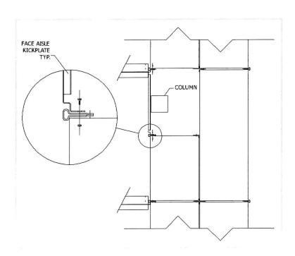
If the column cannot be totally hidden between shelving, then an extension is made in order to adjust the kickplate. The assembly detail is shown below.
