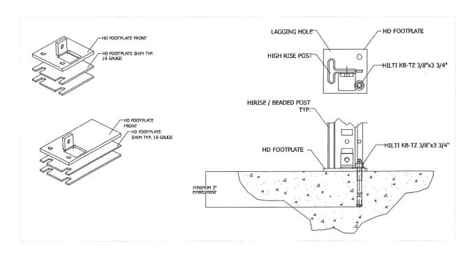
Notice the 3/8" diameter holes in the footplates: the side holes for anchoring and the center hole for shimming.
