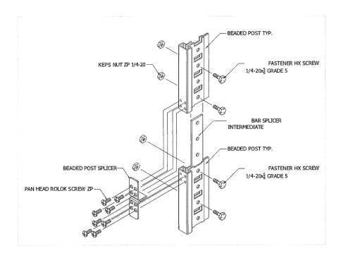
Below is the corner post splicer, used to connect corner angle posts on the ends of rows.
