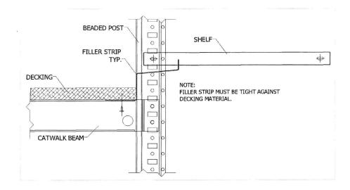
Below, the drawing shows the filler strip installation when corrugated deck is used.
