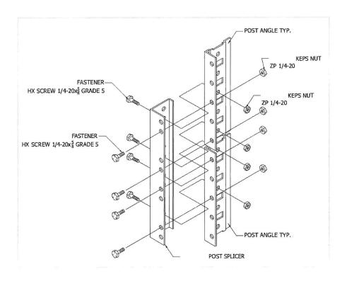
The angle post back-to-back splice is bolted between two angle posts, as shown below.
