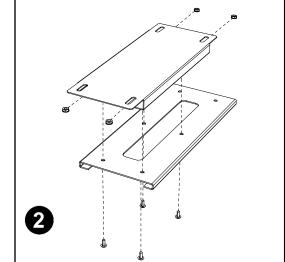
Use supplied (4) 94383-53 screws and (4) 94394-71 nuts to attach mounting plate and keyboard arm to upper cabinet. Insert bolts through keyboard mounting plate and tighten nuts from inside cabinet (4 places). Refer to keyboard instructions to install the rest of the keyboard tray.
